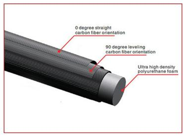
During the heat curing process the 90 degree orientation and the 0 degree orientation fibers work together to ensure there is no displacement resulting in a perfectly straight and strong shaft even after curing.
